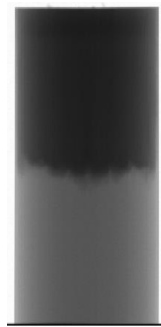
Figure 7.7 – X-ray projected image of a monolith. At the top, the black pixels identify the region where the high density washcoat is deposited. At the bottom, the grey pixels show the uncoated area.
