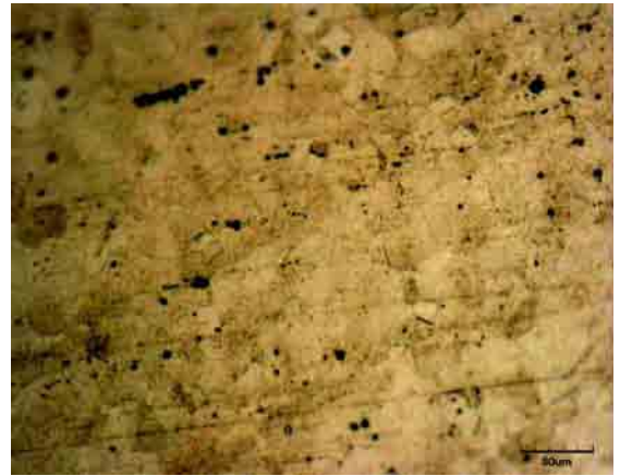
Figure 44 Confocal microscope images for Pd-8at%-0.5at%Cu annealed, etched in 30% nitric acid at 70°C
