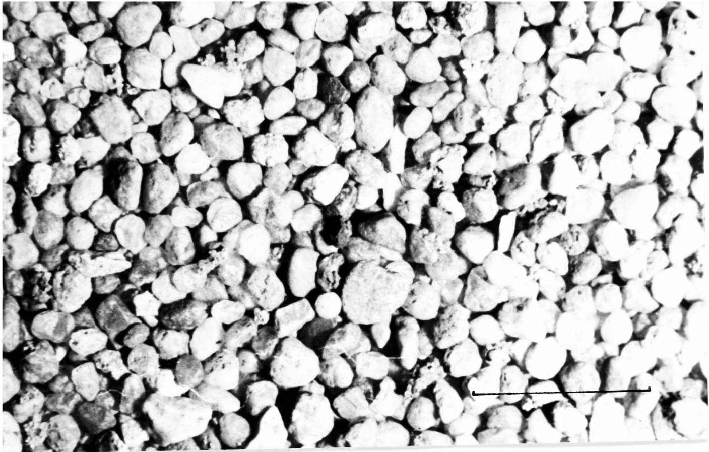
Figure 7. Photomicrograph of sample of coarse sand from Messingham. Millet seed grains of Bunter sand and subangular flints are evident.
