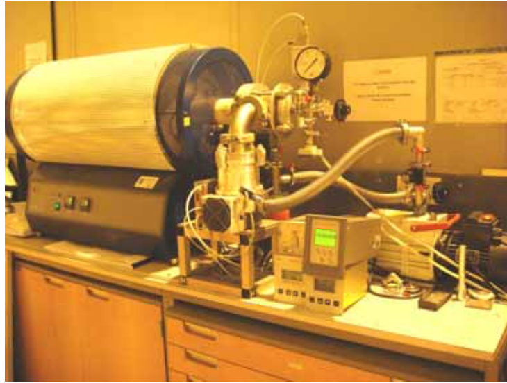
Fig. 3-2 Vacuum furnace for annealing mild steel cans which are used for powder HIPping to get rid of impurities inside.
