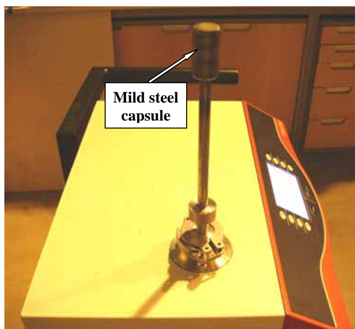
Fig. 3-1 A photograph of leak detector for the checking of capsule's sealing quality.
