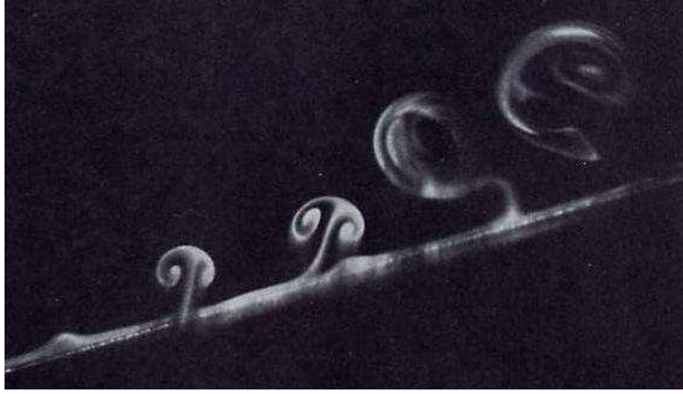
Figure 1.1: Cross-sectional flow visualisation showing pairs of counter-rotating Görtler vortices at \psi = 15^\circ (Kobayashi & Izumi [26]).
