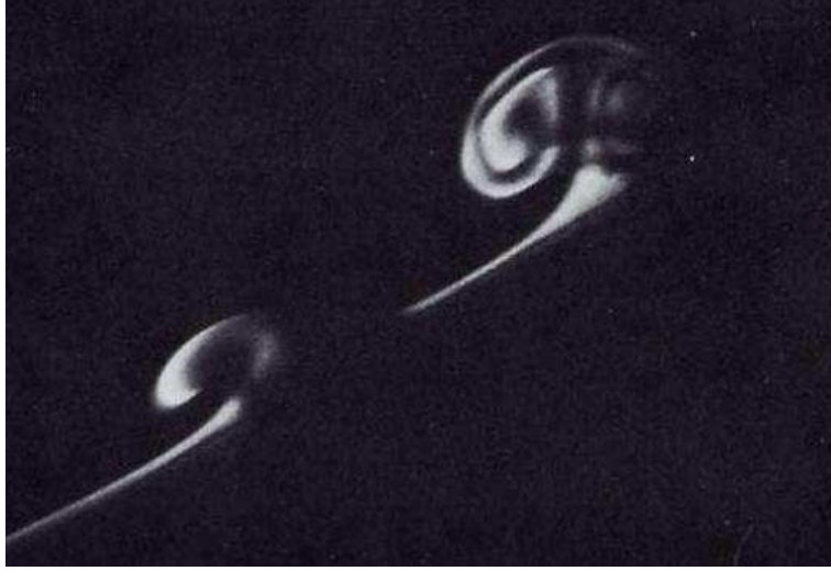
Figure 1.2: Cross-sectional flow visualisation showing co-rotating crossflow vortices at \psi = 30^\circ (Kobayashi & Izumi [26]).
