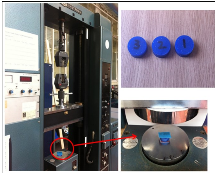
Figure 3-6 Compression test for A90 Polyurethane specimen
