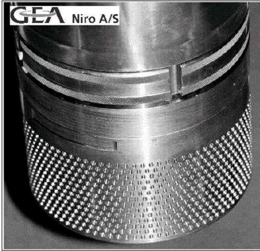
Figure 1.1: Photograph of a prilling can, courtesy of GEA Niro A/S.
