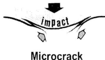
Figure 16 - Formation of micro-cracks on a shot peened surface. Taken from [96].
