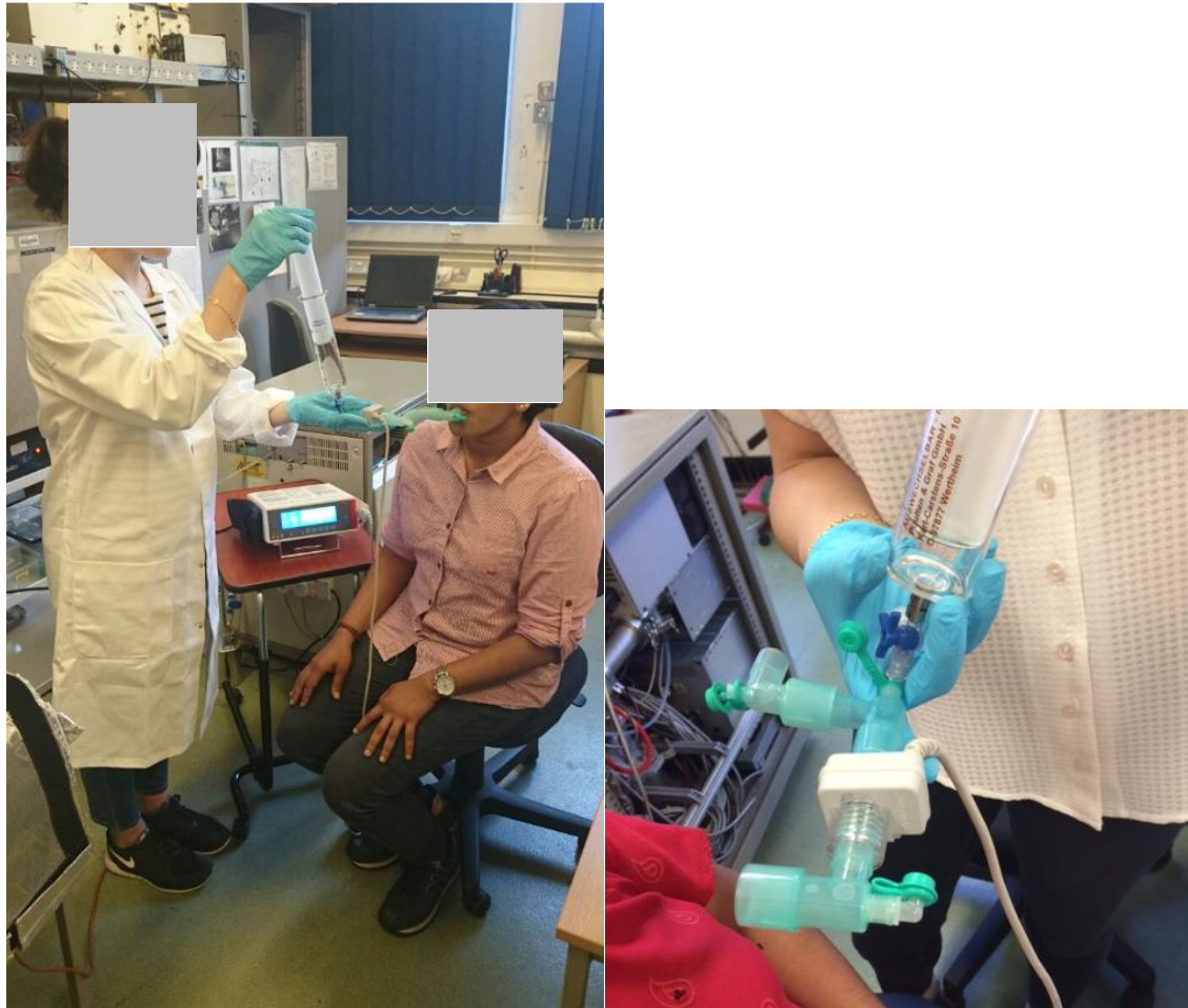
Figure 3.11 Photograph showing a healthy volunteer giving a breath sample. In the right, the photograph shows a close up of the capnostat sensor with the airways adapter coupled to the respiratory breath tubing.
