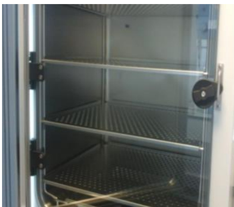
Fig 4.6: Incubation – 37 °C at 5% CO 2 and 98% relative humidity for 24 hr.
