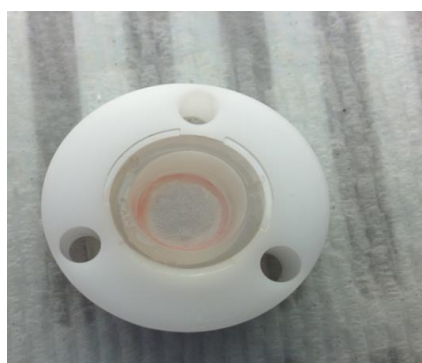
Fig 4.7: Donor Compartment with the skin insert.
