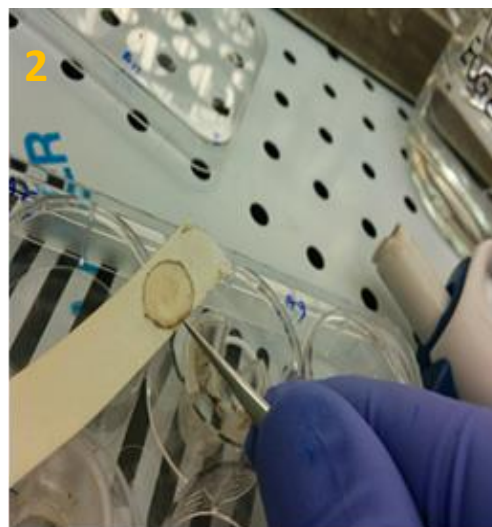
Fig 5.3: Tape stripping with the help of 3M adhesive tape (Pic 1-4).
