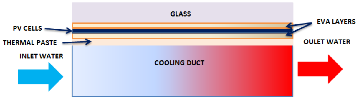
Figure 5-8 schematic diagram for the cooling system
