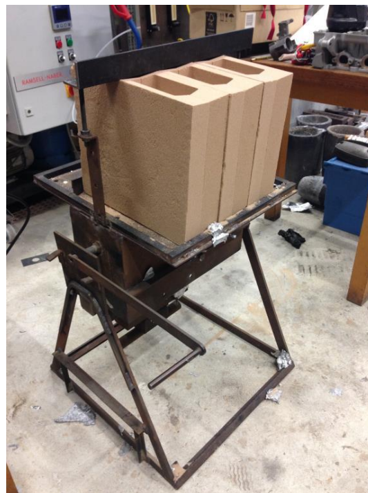
Figure 3-4 the rollover device used for minimise the formation of shrinkage porosity in the casting
