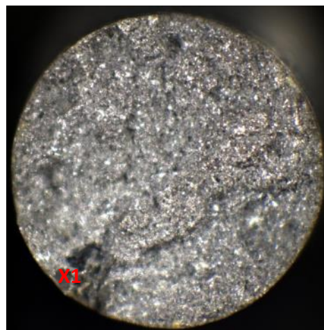
Figure 4-69 Fracture surface of tensile test bar No. 15 of the heat-treated 2L99+ 0.4 wt.% Mo casting; X1 the area shows in Figure 4-70.
