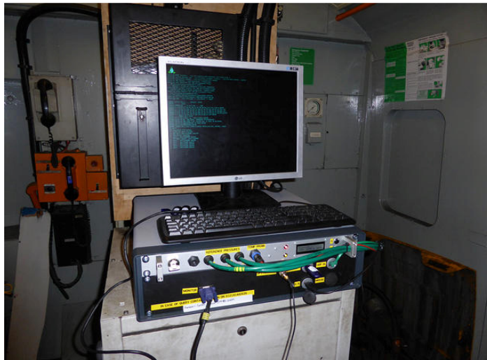
Figure 9.10 - Onboard PC mounted on electrical equipment storage cabinet.
