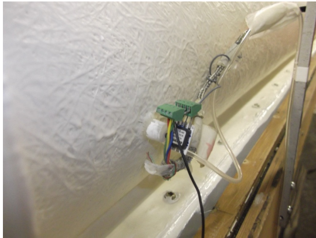
Figure H.5 - Pressure transducer mounted inside nylon block glued to outer surface of tunnel.
