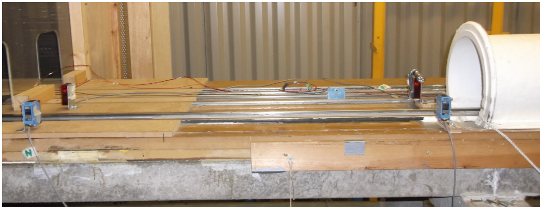
Figure 6.13.1 - Two pairs of light gates spaced 1 m apart, with LED light source on first (RHS) light gate.
