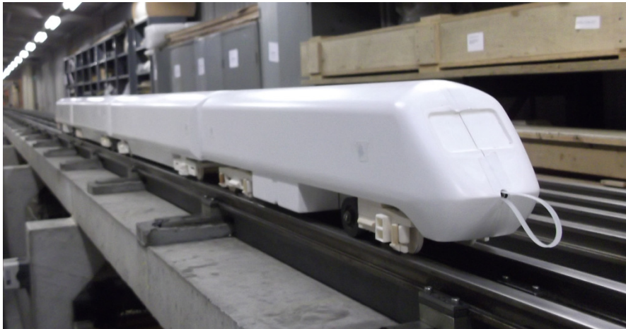
Figure A.3 - Rear of HST model showing loop that attaches to retracting rope (via a rubber band).
