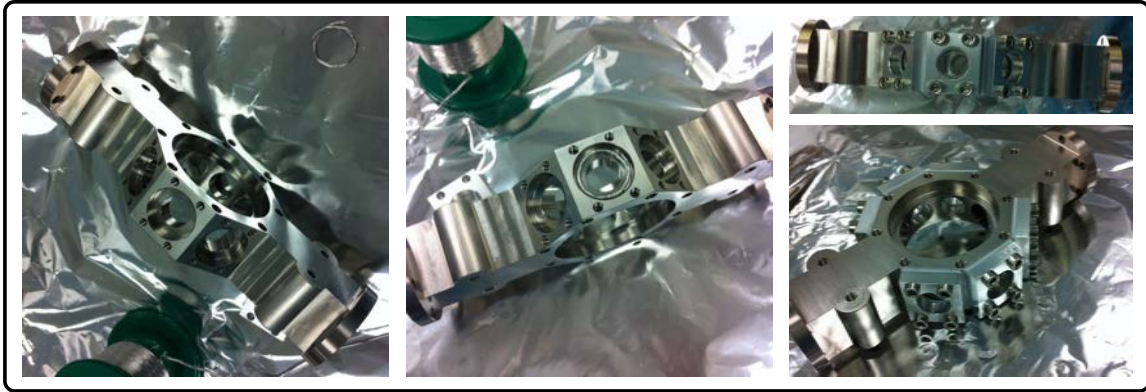
Fig. 5.5 Photographs showing the indium sealing technique for securing vacuum chamber windows. Left: The prepared atomic chamber with the indium ring shown in the top right. Middle: The indium seal placed upon the chamber in preparation for sealing the window. Right: The chamber after all windows had been sealed together with the compression flanges.
