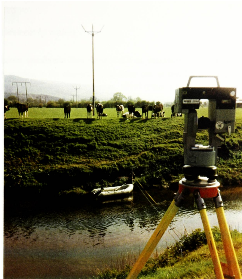
Plate 3.1 Water surface slope surveying, using the EDM (at Pool Quay).
