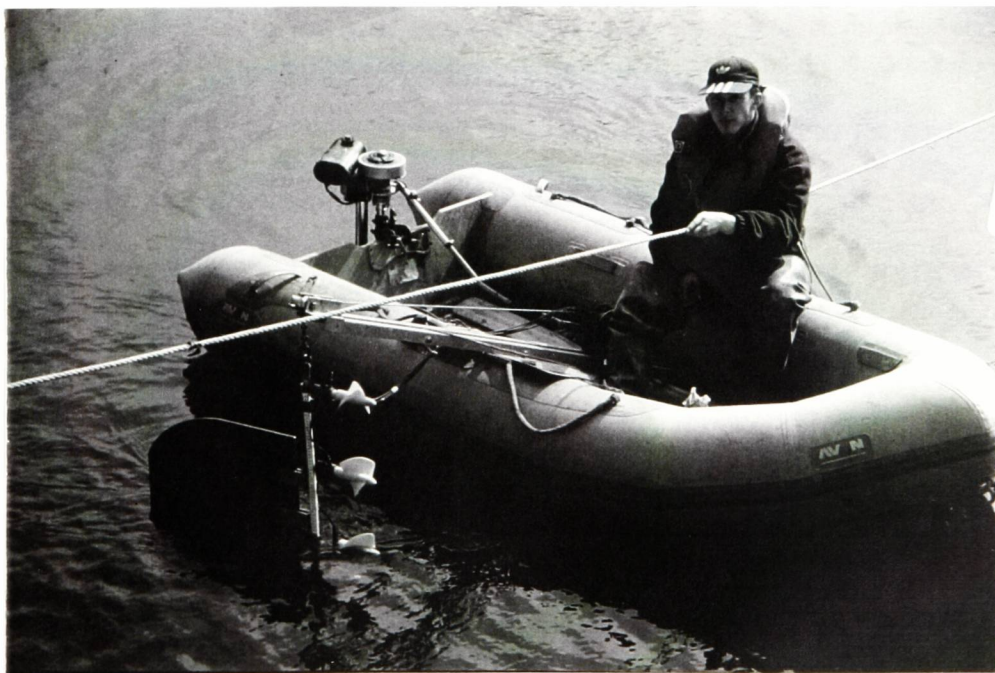
Plate 3.4 Flow measurement from a boat (at Bewdley) (photograph by D. M. Lawler).
