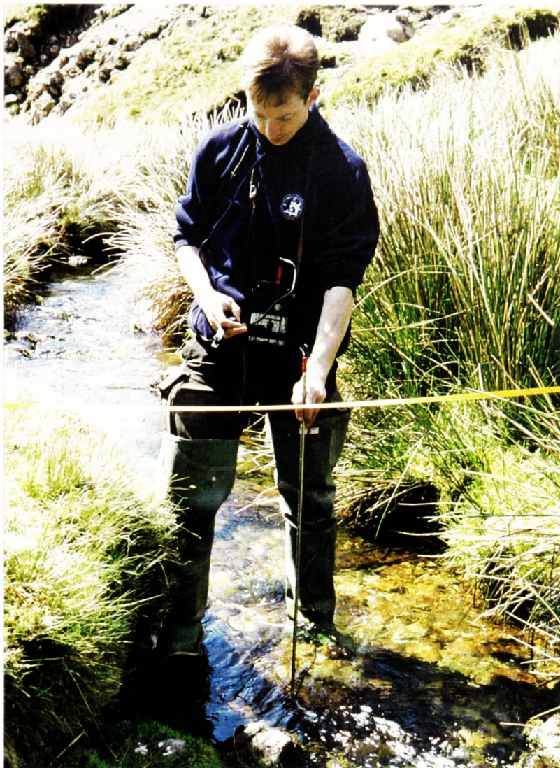
Plate 3.3 Flow measurement by wading (at Upper Hafren 3).
