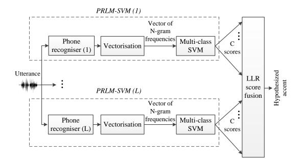
Fig. 2.1 The SVM scores produced by L parallel PRLM-SVM systems are fused using LLR
