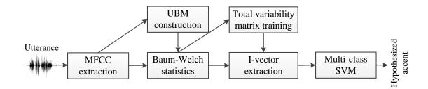
Fig. 2.2 A summary of different stages of i-vector extraction process
