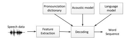
Fig. 3.1 Diagram of a simple speech recogniser
