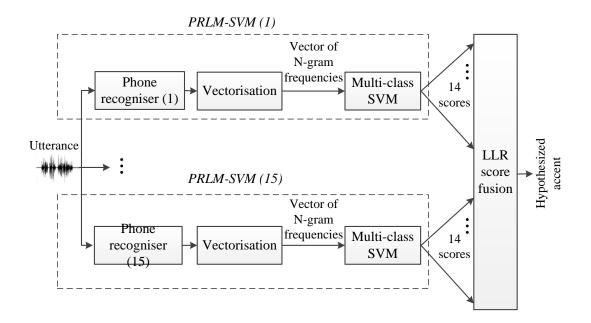
Fig. 6.1 Using LLR to fuse the scores from 15 parallel PRLM-SVM AID systems
