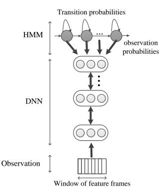
Fig. 3.7 Structure of a DNN-HMM system [5]
