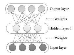
Fig. 4.2 A multi-layer perceptron with one hidden layer
