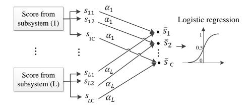
Fig. B.2 Fusion the scores from L subsystems with C classes using LLR approach
