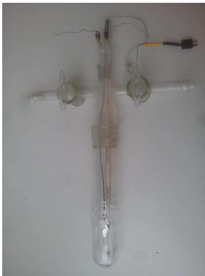
Figure 2.23 Finished constructed air-sensitive A.C. impedance containment rig
