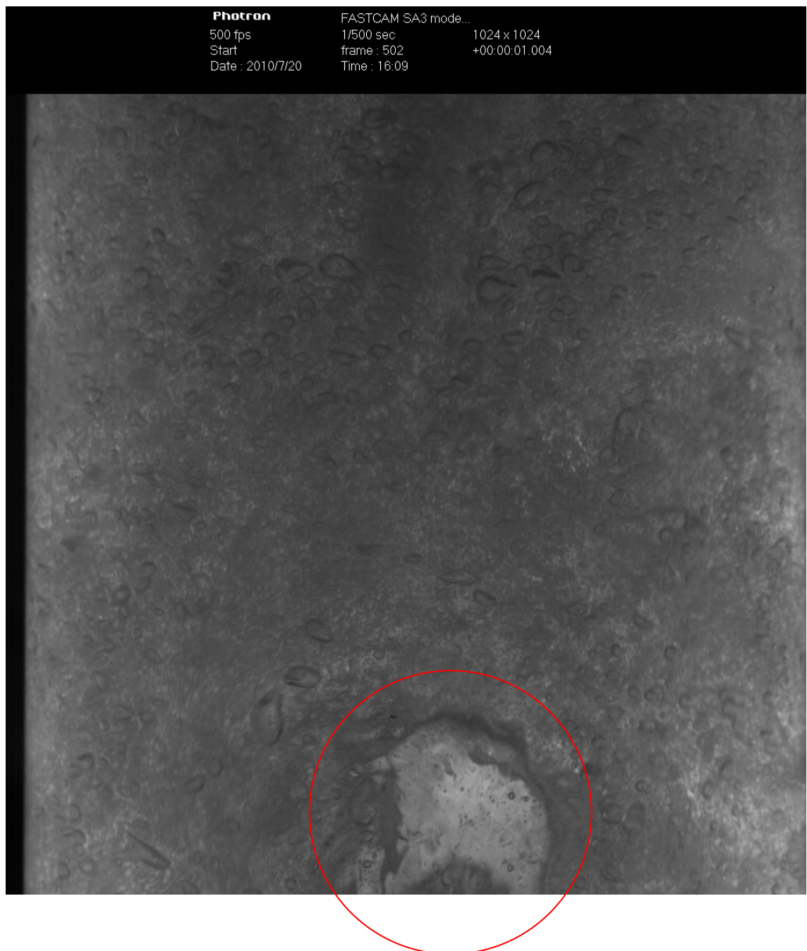
Figure 4.4 Image of heterogeneous flow of air-water column for flow visualisation experiment 2; superficial gas velocity 6.1 cm/s, 1 kg of dissolved sodium chloride. Internal column diameter of 144 mm. TIFF image belongs to file flow_vis_ext_2.avi. Red circle indicates air void within its perimeter.
