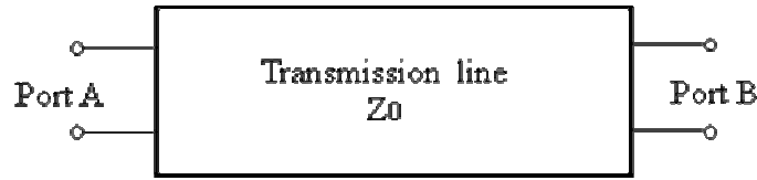
Figure 2-2. Transmission line model: a two-port network.
