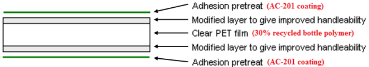
Figure 1.3: The structure of Melinex ® 406R. Diagram obtained from the DTF database.
