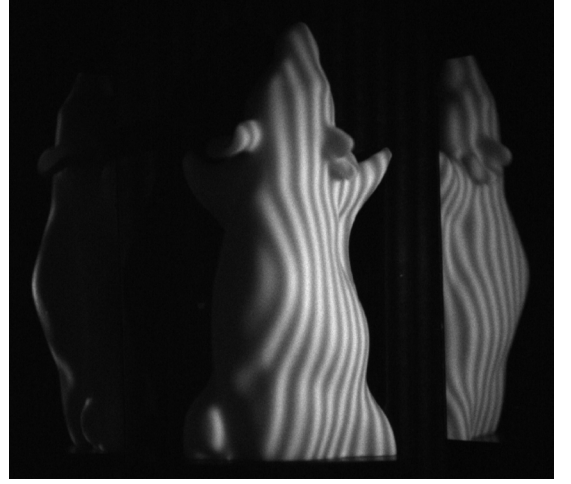
(b) XPM-2 phantom imaged with projector 1 projecting a sinusoidal pattern
