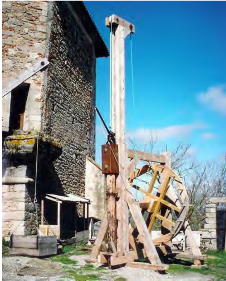
Fig. 1.6: Reconstruction of a medieval pile-driver, Chateau Mezerville, Aude, France.
