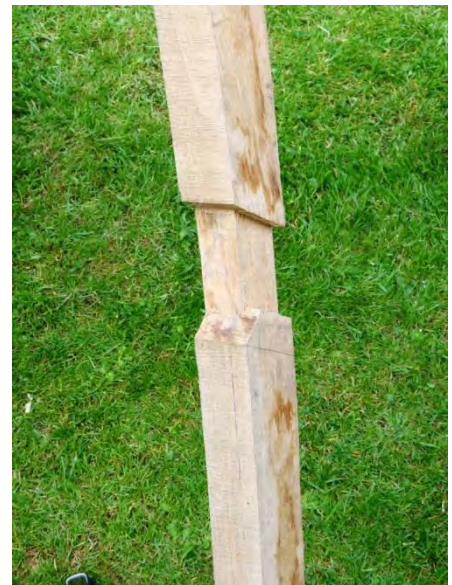
Fig 6.24: Reconstruction of Westminster framing, hammer beam / arched rib configuration; left: cogging of the hammer beam, note also the core is tenoned into the hammer beam; right, the outer laminate of the arched rib; note reduced section where it passes through the hammer beam.
