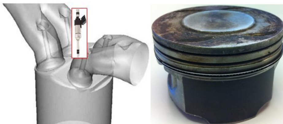
Figure 3-3: Combustion system of single cylinder GDI engine (a) 3D cylinder head diagram, (b) piston
