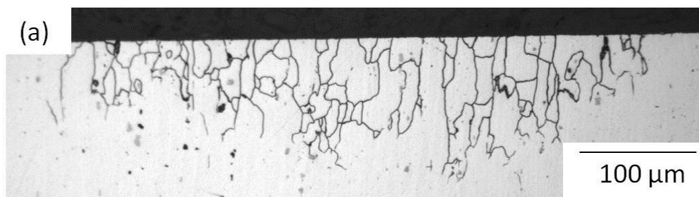
Figure 55 Optical Micrographs from the cross section of AA5083-sensitised parent section after immersion in 1M NaCl for 10 days showing (a) typical intergranular attack up to 100 µm below the surface, which comprised the majority of the attack seen.
