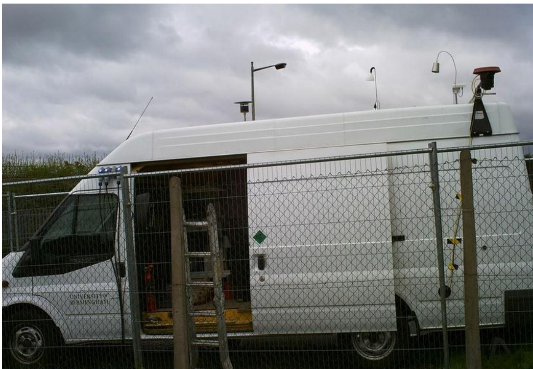
Figure 2.8: The Mobile Laboratory showing sampling inlets of ATOFMS and other instruments during Port Talbot sampling campaign
