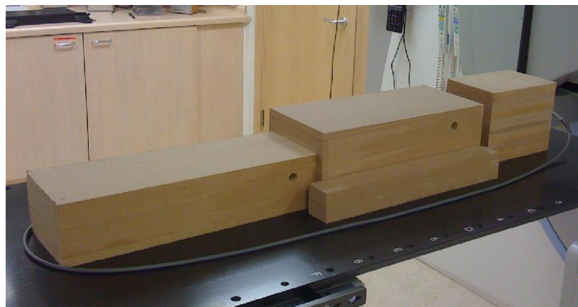
Figure 7.4. Details of the paediatric anthropomorphic phantom used for measurements, distances as marked (mm). Measurements were performed with an NE2571 chamber.
