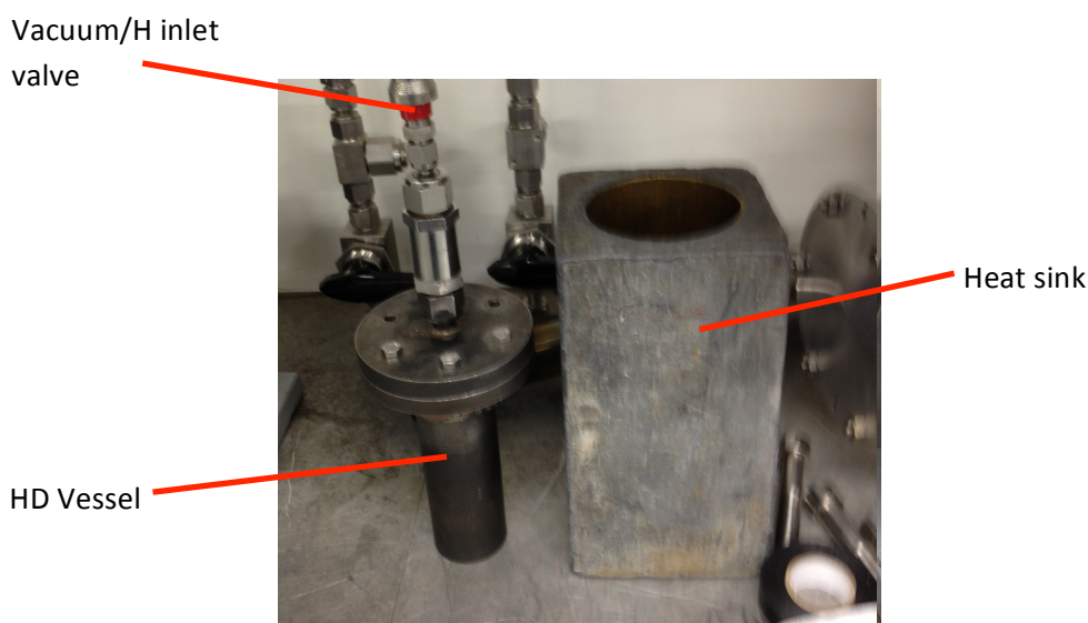
Figure 28 – Image showing the HD Processing equipment used for this project.
