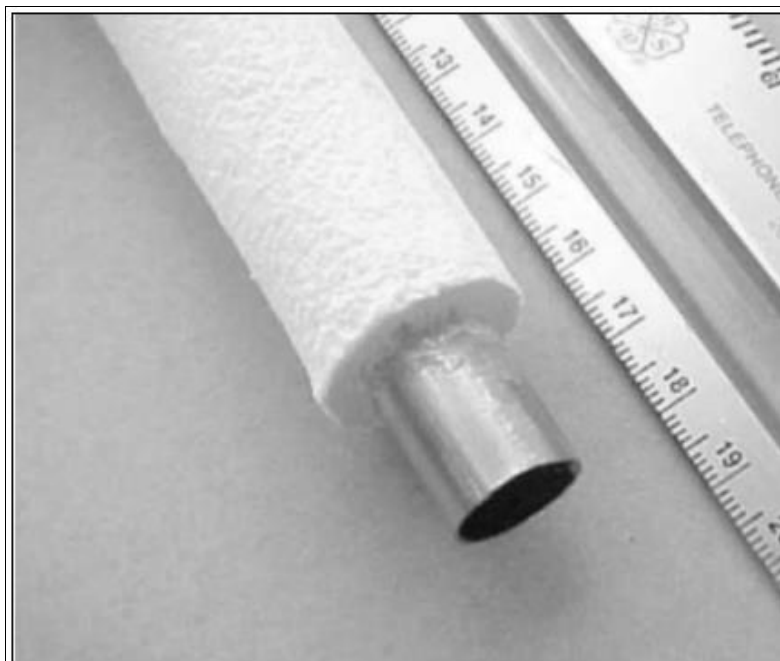
Figure 2.17 Consolidated adsorbent onto tube Marletta et al [45].
