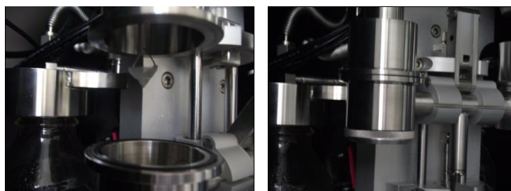
Figure 4.3 Sample container suspended on an extension wire.
