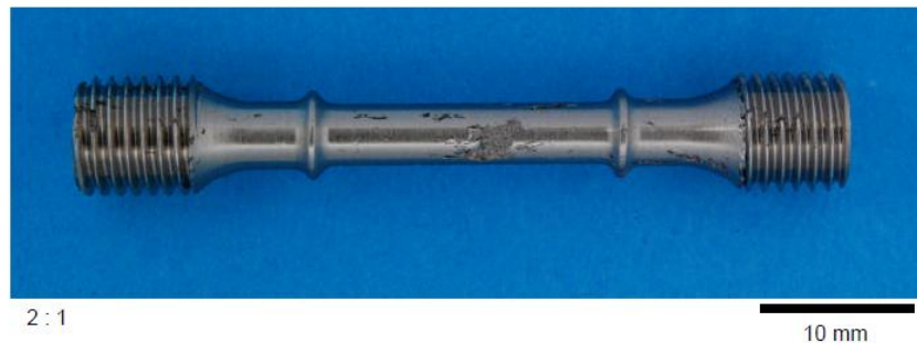
Figure 6.26: Photograph showing SLM-fabricated CMSX486 following HIPping, heat treatment and machining to test specimen geometry. Note the extensive cracking visible along the length of the sample.
