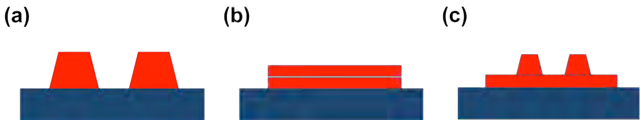
Figure 1.5 (a) Volmer-Weber; (b) Frank-van-der-Merwe; (c) Stranski-Krastanov growth modes.
