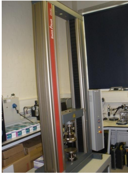
Figure 4.21 The universal material testing machine Z030, Zwick Roell, Germany).
