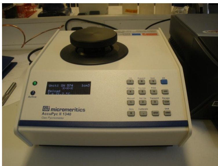
Figure 4.8 Helium pycnometer (AccuPycII 1340, Micromeritics USA).
