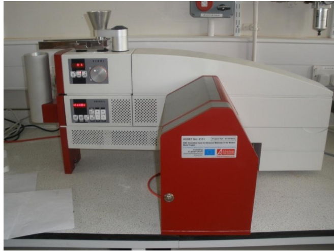
Figure 4.6 Laser particle size analyser (HELOS mode, SympaTec, Germany).
