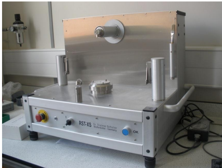
Figure 4.9 The RST-XS ring shear tester.
