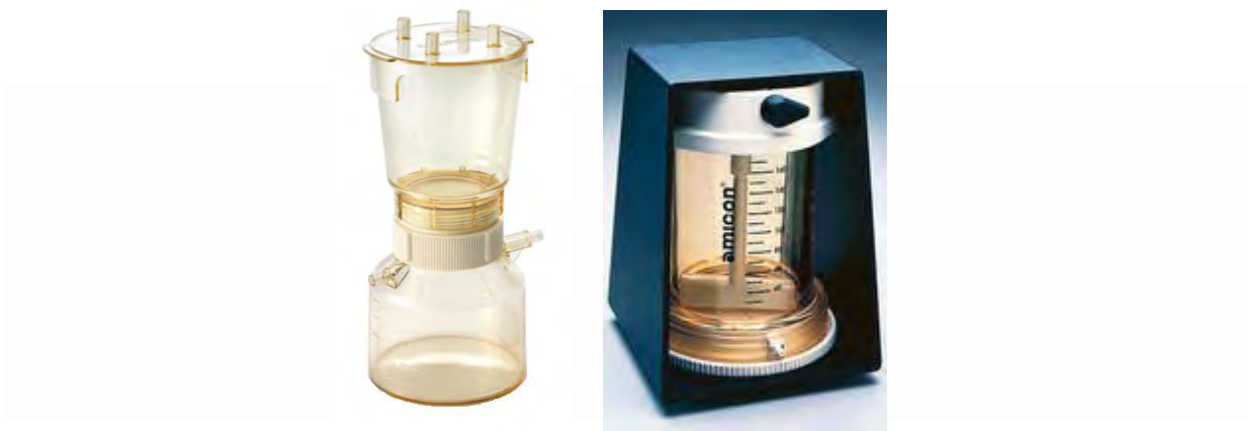
Figure 2.1 Left: millipore sterifil filtration system. Right: Ultrafiltration equipment assembly. Sample is placed in chamber, \text{N}_2 gas is passed over the sample from the top with the filtrate collected from the bottom. The sample is stirred to reduce aggregation as the sample concentrates. Images obtained from Fisher Scientific, UK.
