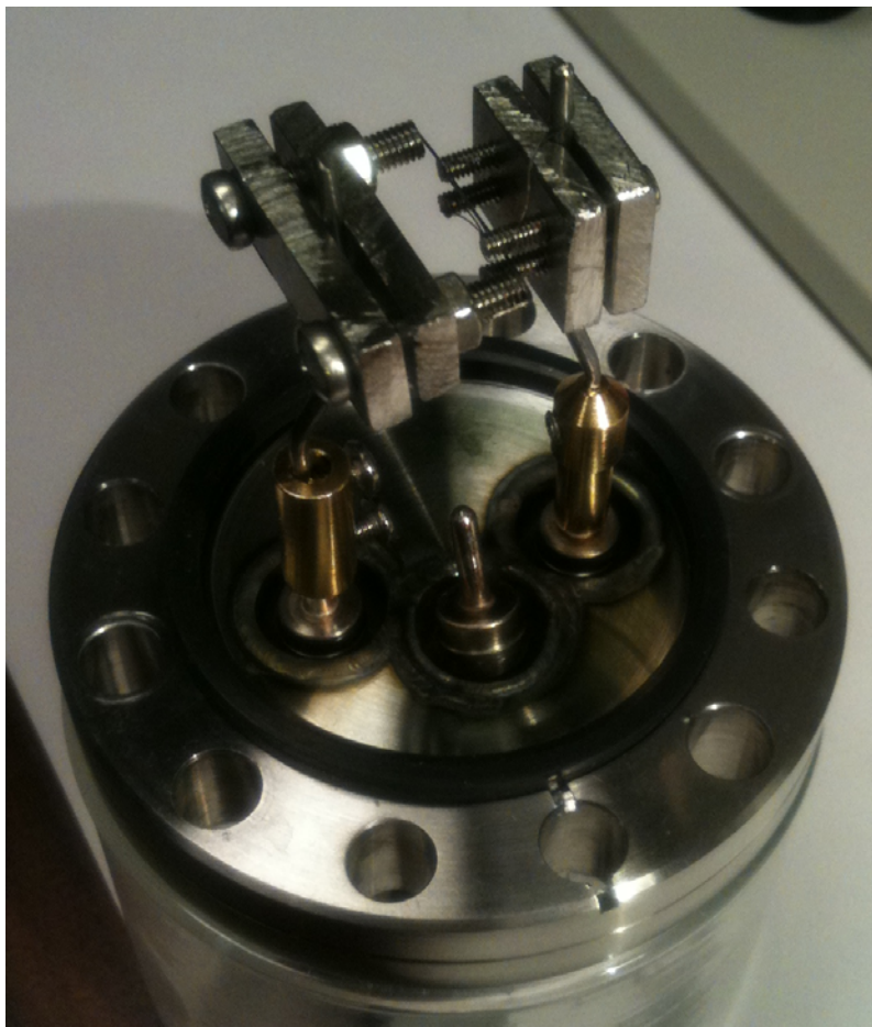
Figure 8.4: Device to clamp and anneal tips for MBE deposition.
