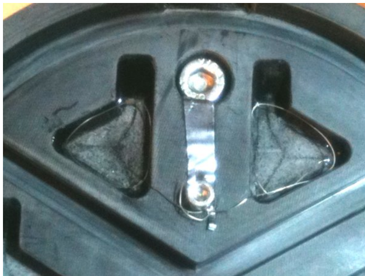
Figure 8.2: High-density polyethylene disk designed with 6 compartments, 2 for etching and 4 for rinsing. This picture depicts the etching compartments, the groove for pouring out liquids, and the etching counter electrodes (immersed tungsten loops).
