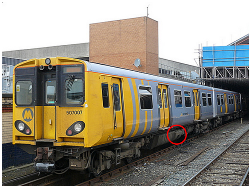
Figure 3.1: Class 507 with equipment rack containing instrumentation highlighted
