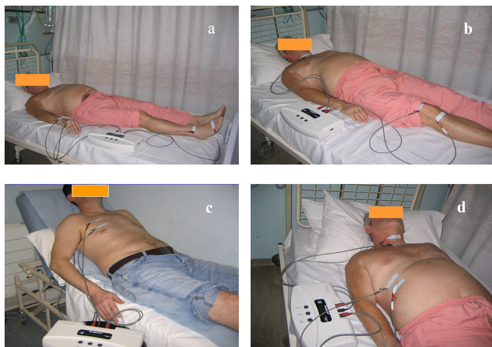
Figure 4.6. Bioimpedance analysis across whole body (a), trunk (b), right lung with electrodes in anterior-posterior position (c) and sternum-rib position (d).
