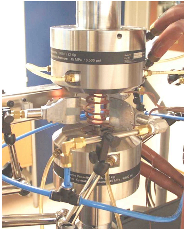
Fig.2.8 MTS 810 servo-hydraulic testing machine in SIEMENS Industrial Turbomachinery AB in Sweden.
