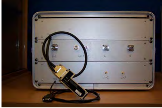
(a) Front view, inputs to three receiving channels and data interface to PC
