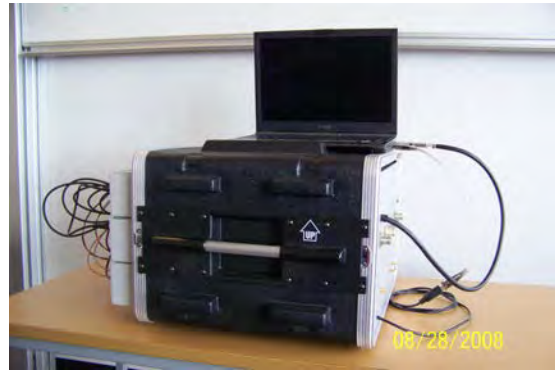
(d) Fully connected microwave receiver with a laptop for data collection
