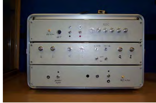
(b) Rear view, three pairs I/Q outputs and other inter-connection ports
