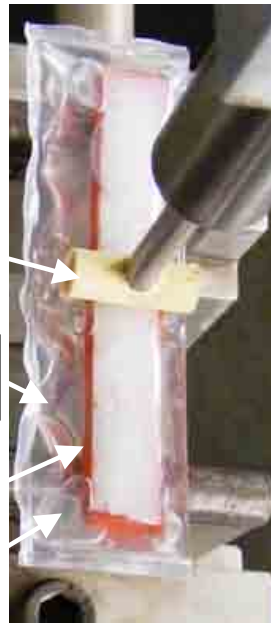
Figure 4.46 Flexural creep test sample.
