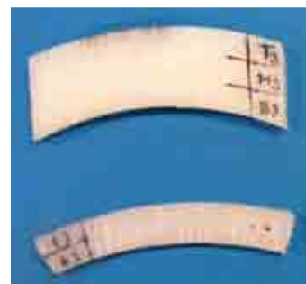
Figure A.1 Samples for the density test of DN250 pipes, (top) SDR11 and (bottom) SDR21.
