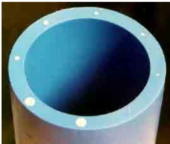
Figure 2.30 Location of planar flaws of different sizes (Troughton, 2001).
