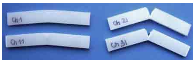
(a) (b) Figure 5.77 (a) Unnotched and (b) notched Charpy impact samples after failure.
