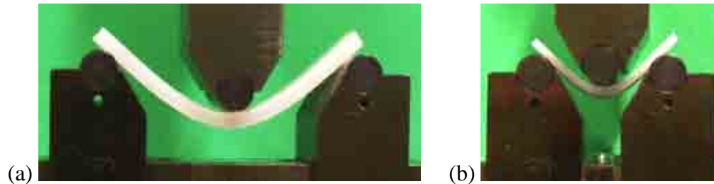
Figure 5.75 The test arrangement in 3-point bending for (a) 4.2mm and (b) 2.2mm thick samples.
