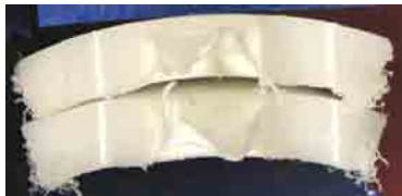
Figure A.43 Cross-section of broken DN250 SDR21 joint sample 5/2.
