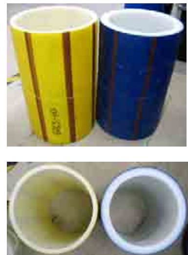
Figure A.4 DN250 SDR21 and SDR11 pipe sections used to produce butt-fusion joints: (a) side and (b) top view.
