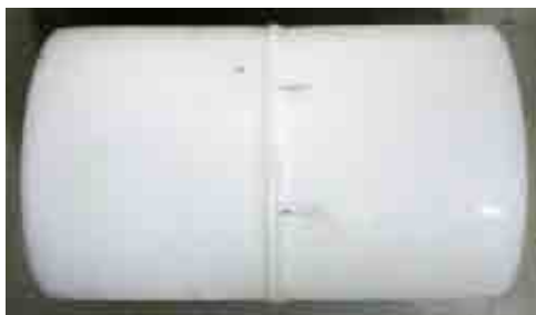
Figure A.8 Butt-fused pipe with a bead.
