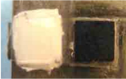
Figure 6.13 The cross-section of the debonded sample showing the broken chip after the pull-off test on a HMA1-silicon chip sample.
