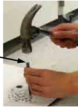
Figure 4.27 Cutting out the circular chip from the HMA sheet using a punch.
