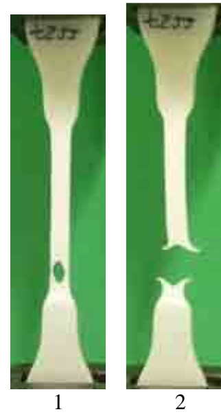
Figure 5.51 Profiles of the SC&SSQ/0/90 sample during characteristic stages of the tensile test.
