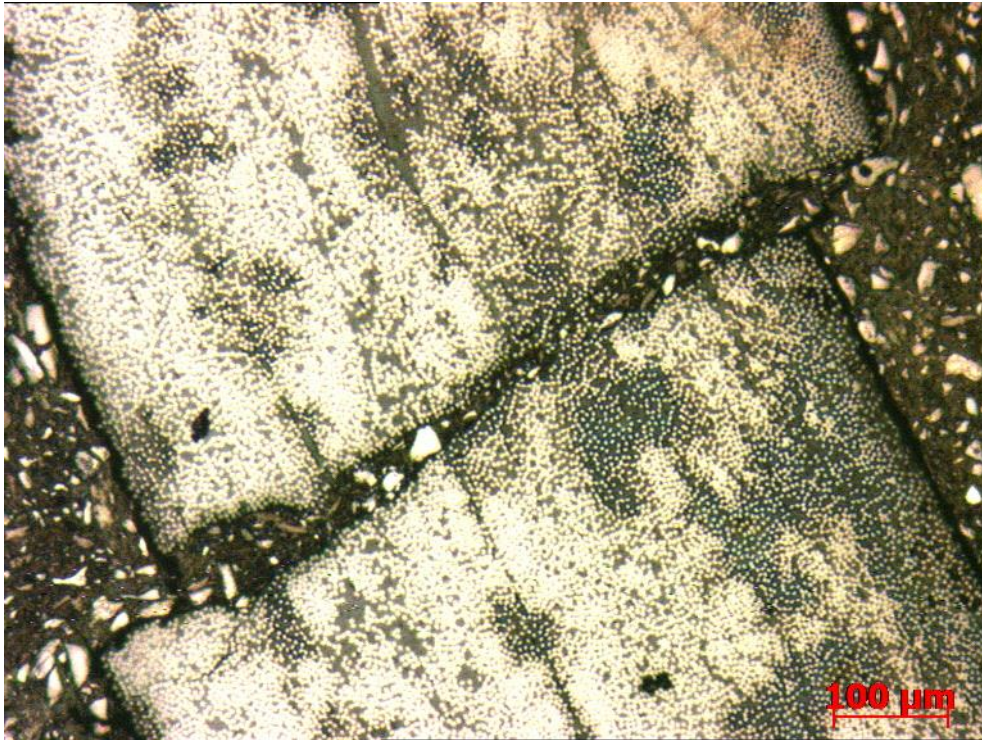
Figure 8.13: Micrograph of crack found in shaft 0-I
