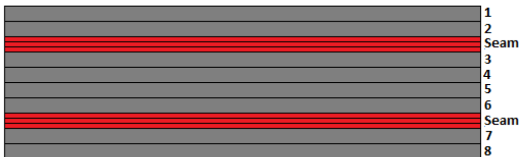
Figure 3.1: Schematic diagram showing the locations of the seam and ply numbers in a panel.
