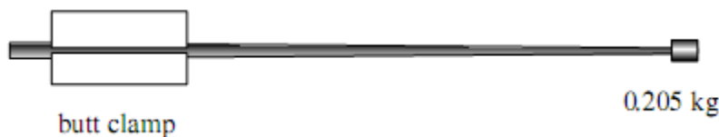
Figure 1.8: Schematic diagram showing the frequency testing method.
