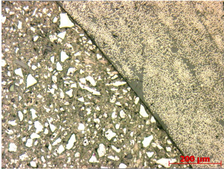
Figure 8.8: Micrograph of seam found in shaft 0-II.
