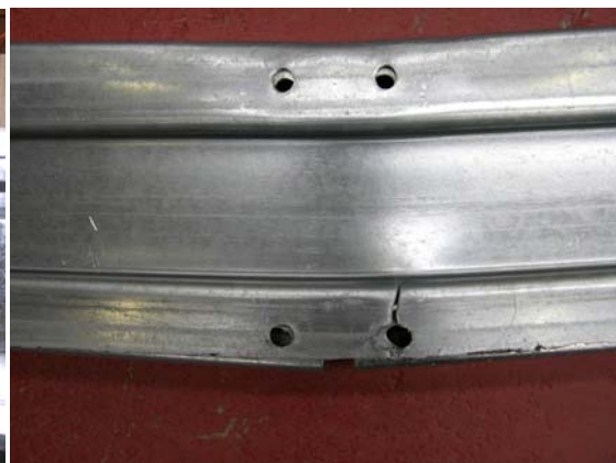
(b) Tension fracture failure in sleeve section (failure mode 2)
