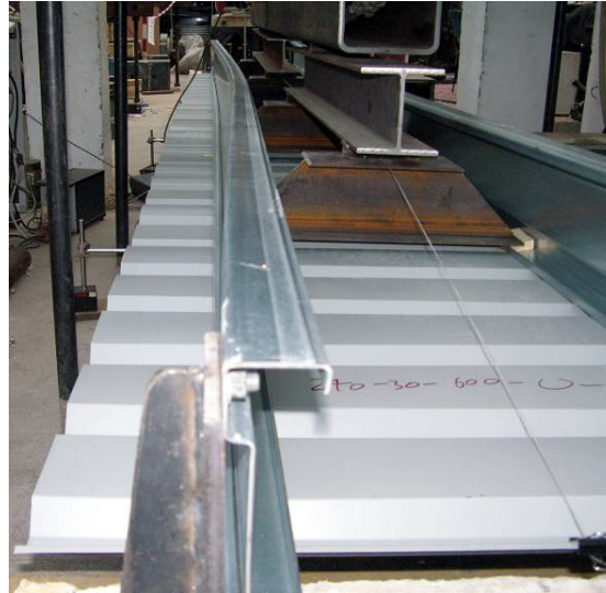
Figure 5-11 Typical deformation of sheeted purlin with unrestrained compression flange
