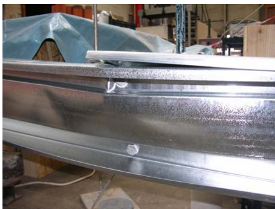
(a) Local buckling in the outer web of purlin section (failure mode 1)
