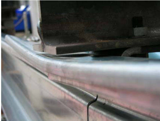
(c) Local buckling in the compression flange of sleeve section (failure mode 3)
