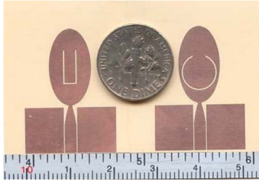
Fig. 2.37 CPW-fed compact elliptical monopole UWB antennas integrated a U-shaped slot and a C-shaped slot, respectively [35]
