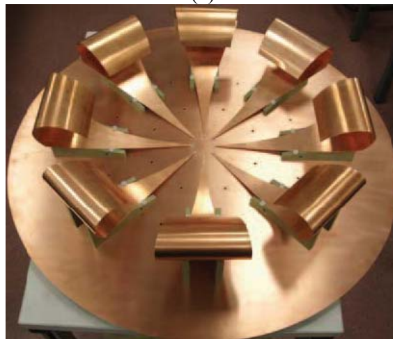
Fig. 2.5 (a) Architecture of the wideband antenna with reconfigurable pattern notch; (b) Prototpye of the TEM circular array [4]
