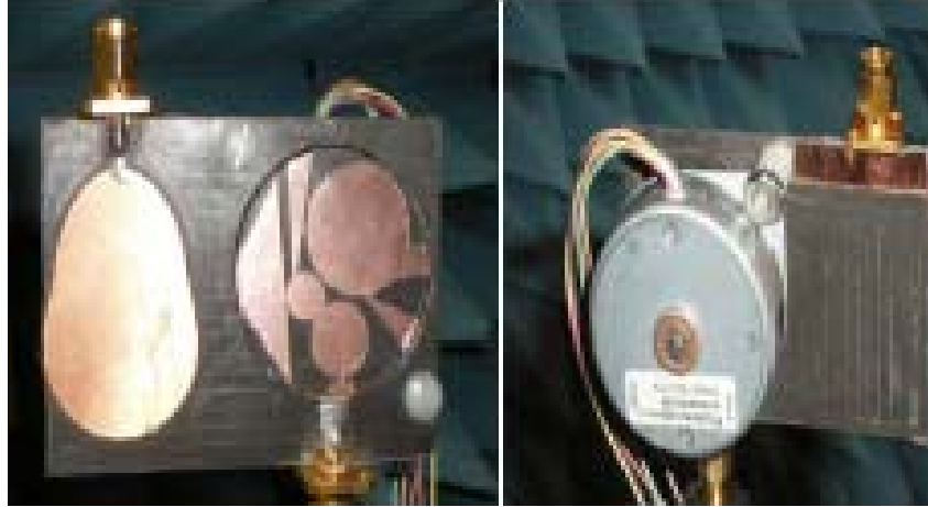
Fig. 2.22 The fabricated prototype combined with a UWB sensing antenna and a frequency reconfigurable communicating antenna. [21]
