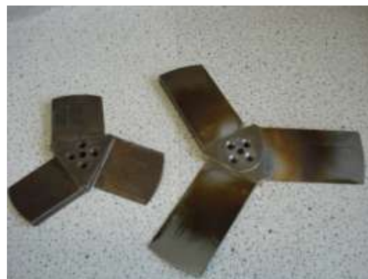
Fig. 4.4. Three-blade impellers for the small and large bowls used in study.
