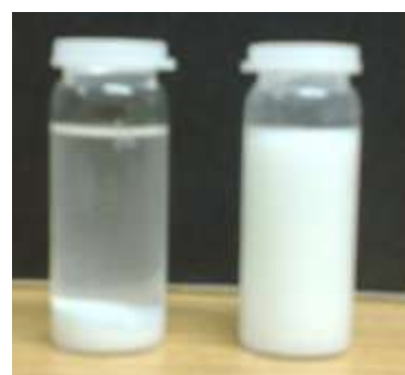
Fig. 2.3. Lactose in propan-2-ol suspensions; without sonication (left); 1 min after sonication for 3 min (right).
