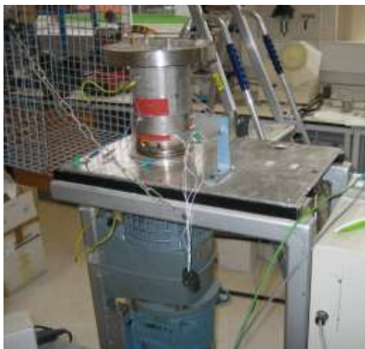
Fig. 4.3. Small bowl with lid shown resting on bearings driven by the 7.5 kW motor.
