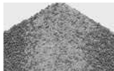
Fig. 4.7. Segregation of fine (light grey) and coarse (dark grey) particles.
