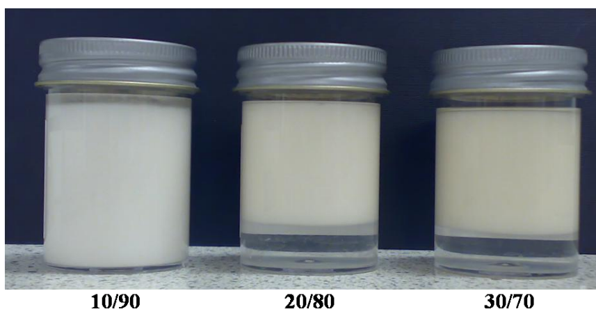
Figure 4-9: Effect of the oil concentration on the O/W emulsions prepared at pH 2 with 2 wt/wt% Aerosil 200 – after 1 month.
