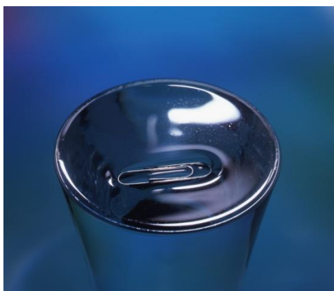
Figure 2-1: Mechanical point of view of interfacial tension – Paperclip at the surface of water – photograph provided by Kruss ( personal communication ).
