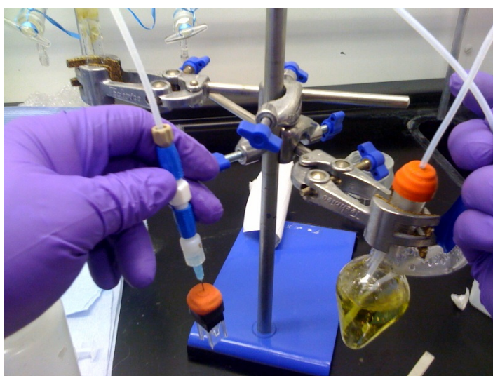
Figure 3.1 Solution transfer via syringe from flask into a plastic cuvettes for Mo(V) solution.
