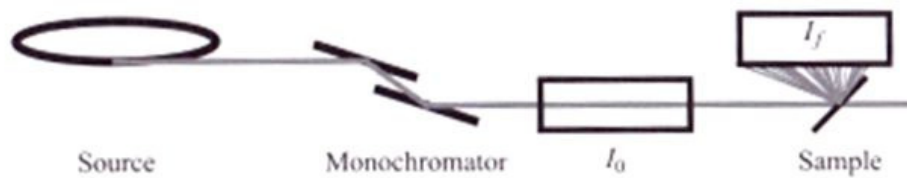
Figure 2.20 Fluorescence XAFS experimental configuration [121].
