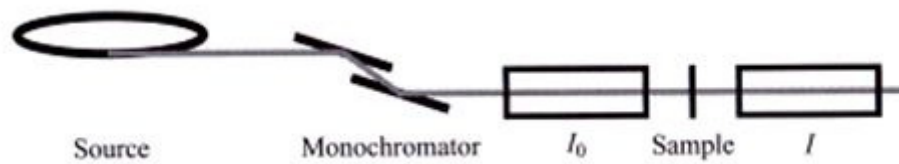
Figure 2.19 Transmission XAFS experimental configuration [121].
