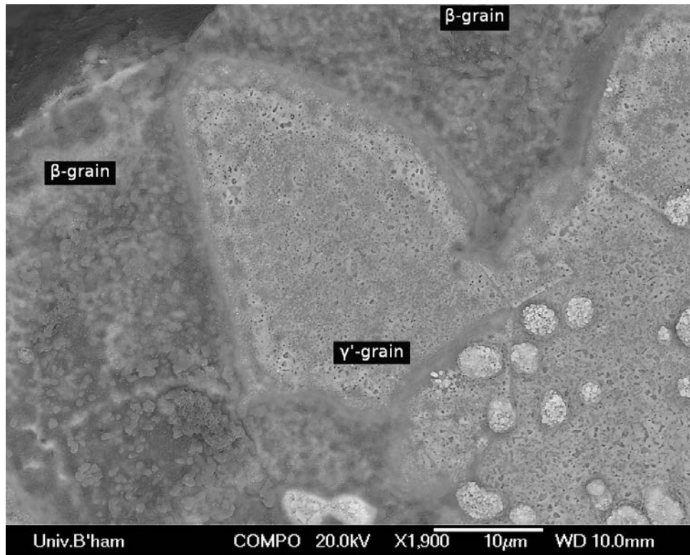
Figure 4.21: BSE micrograph showing the composition of the underlying bond coat phases, through the oxide layer.
