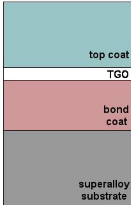
Figure 2.10: Schematic cross-section through a thermal barrier coating. Showing all the layers as discussed above.
