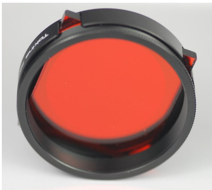
Figure 44 636nm narrow band interference filter and its spectral absorption.
