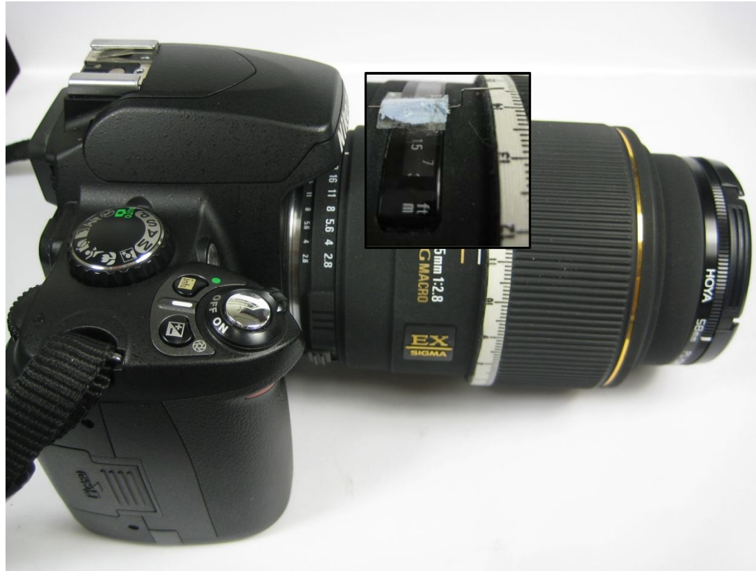
Figure 31 Location of the plastic scale attached around the lens barrel in the camera and the piece of wire used to register the focus shift.
