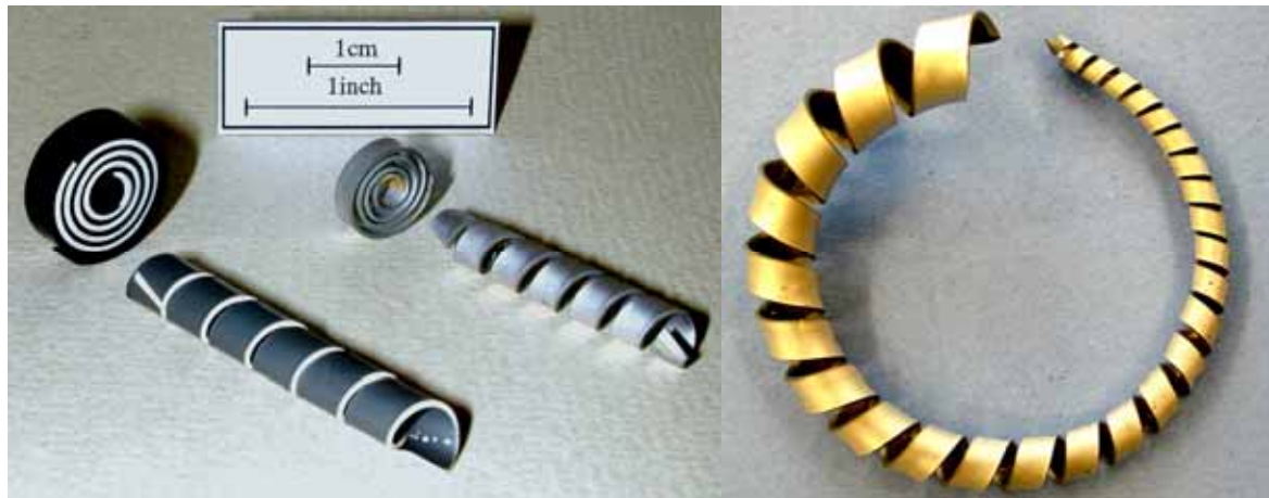
Figure 4.20: Examples of net-shaped helimorph actuators manufactured using a viscous plastic processing route. Pictures courtesy of Su, Pearce et al (21, 27, 28) , 1998.
