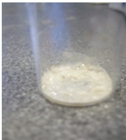
Figure 6.29. Crystallised sample for reaction condition of 300 °C and 80 bar; in case 3.
