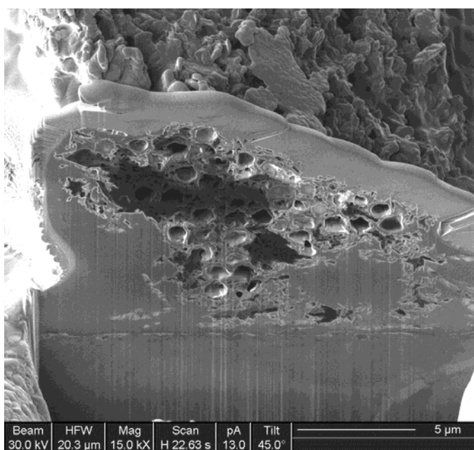
Figure 3.13 FIB induced secondary electron image showing the cross section view of an aggregated structure after calcination at 550 °C.
