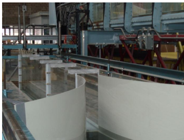
Figure 3.10 The 3 m x 0.15 m test section of the larger flume.
